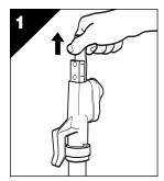
Before assembling appliance, remove two screws from the connector assembly. Remove cardboard insert by pulling upward.
